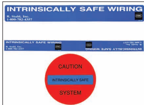
Figure 12. Intrinsically safe wiring shall be identified as such using labels placed at no more than 25 foot intervals. R. STAHL recommends that when using zener diode type safety barriers that the I.S. ground conductor be labeled as well.
