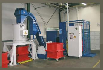
▲ Swarf processing system, consisting of: Lifting and tipping unit for loading a Type RS 300 E swarf crusher and a scraper conveyor to in-feed a Permolex-Polar Type K 51 centrifuge. The crushed and dried swarf is discharged into on-site container.
