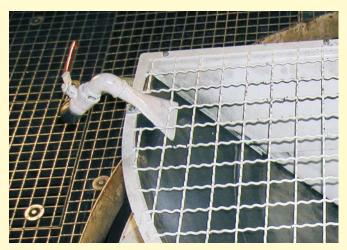
▲ The flushing system is necessary to prevent some swarf types from sticking in the feeding hopper and is designed to be connected to the pumped coolant supply. A flushing nozzle provides a regulated coolant flow into the feeding hopper, which flushes adhering swarf into the centrifuge bowl. For cast iron swarf the flushing device is necessary due to cast iron and coolant's congealing nature.
