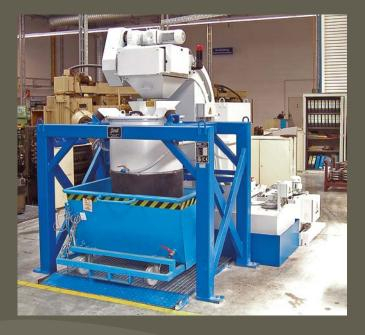
▲ A Permolex-Polar type K 40 K centrifuge, which is loaded by a scraper conveyor and discharges the dried swarf into a container, placed below.
