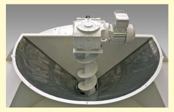
▲ The metering auger in the in-feed hopper of the centrifuge ensures the constant and regulated feeding of swarf into the centre of the centrifuge bowl and allows the hopper to accommodate small surges of swarf. The auger is designed to prevent blockages but if they occur the auger automatically changes rotational direction a number of times to free the blockage or to stop.
