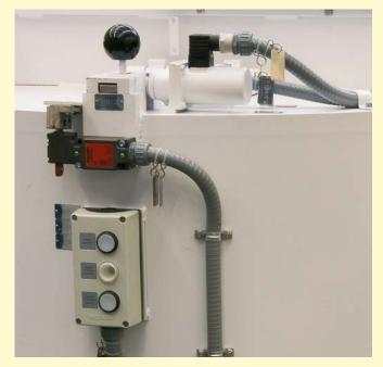
▲ A hinged maintenance inspection access lid interlock, is actuated by a solenoid, permitting access only when the centrifuge bowl monitored rotation has completely stopped. This safe condition of the non rotating bowl is indicated on the control panel as "cover opening possible". The solenoid locking is released via a pushbutton and permits the opening of the access lid. In the standard version this maintenance lid is bolted to the centrifuge casing.
