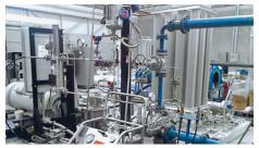
In the LNG processing plant at Cacimbas, **Brazil**, 238 pumps are applied. 75 % of them are equipped with EagleBurgmann seals. For pumping C2+, Sulzer type CAP8 80-430 pumps are installed. Shaft seals are EagleBurgmann API type C seals. Configuration 2CW-CW, piping plans 13, 21, 52 and 65. Liquefied propane is used as cooling fluid for Plan 21 and 52. Operating conditons: p=34 bar (493 PSI), t=-45 °C ... +120 °C (-49 °F ... +248 °F), n=3.565 min<sup>-1</sup>.
