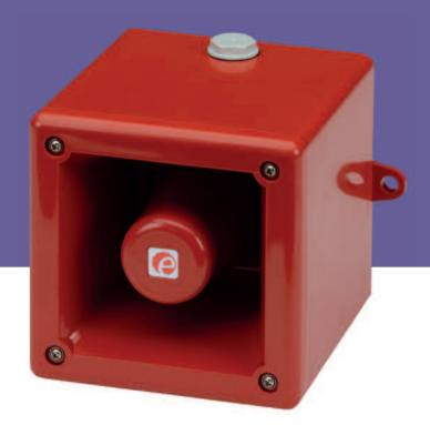
The A105NAX Appello user recordable unit enables the recording of any type of content such as voice or music that can be played back at CD quality output at SPL's of up to 102dB(A) at 1 metre. This content can be reproduced repeatedly, alternating with or without one of the built-in 45 alarm tones. The alarm tone notification has an output of up to 110dB(A) at 1 metre.
